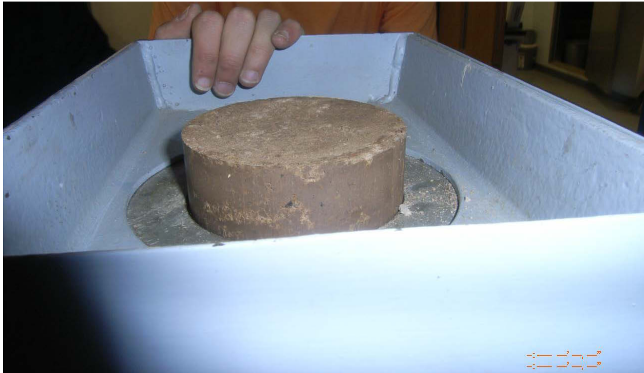
Figure 33: Removal of Compacted Specimen from Mold Using Jack
