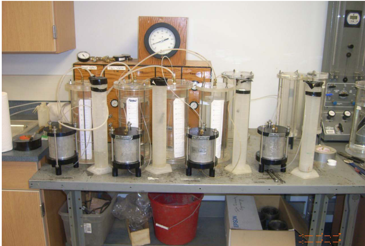
Figure 35: Hydraulic Conductivity Testing
