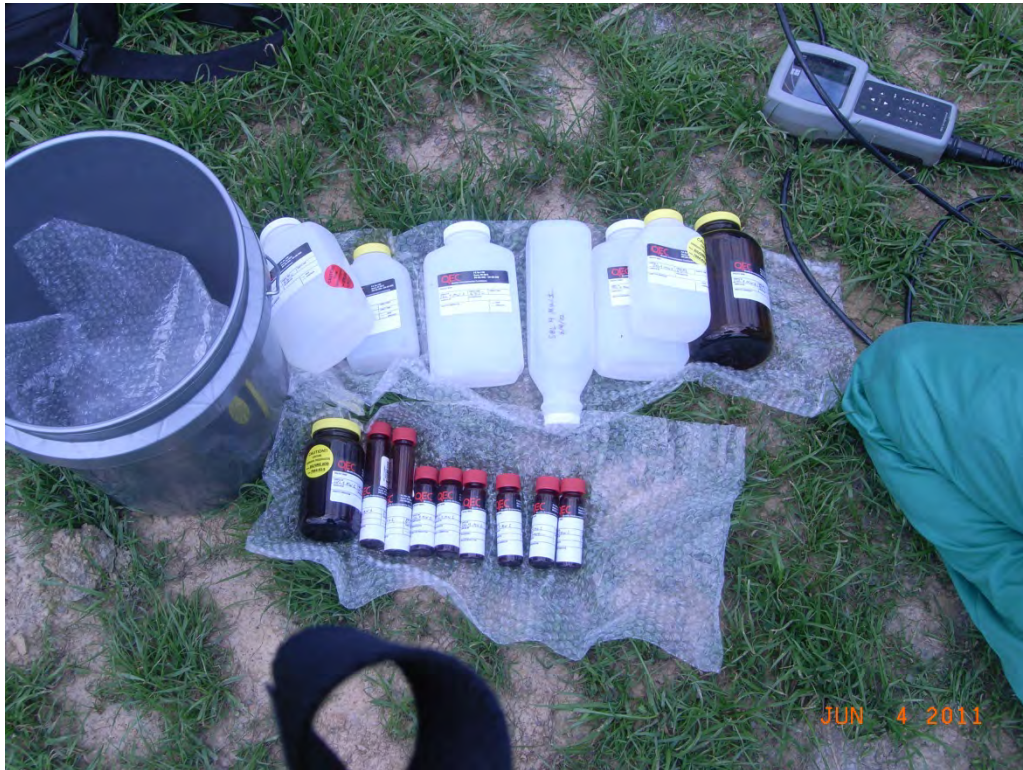
Figure 18: Bottles for Typical Groundwater Sample
