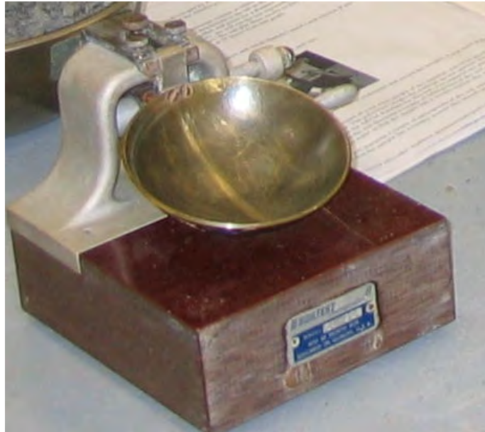
Figure 29: Liquid Limit Device (Casagrande Cup)
