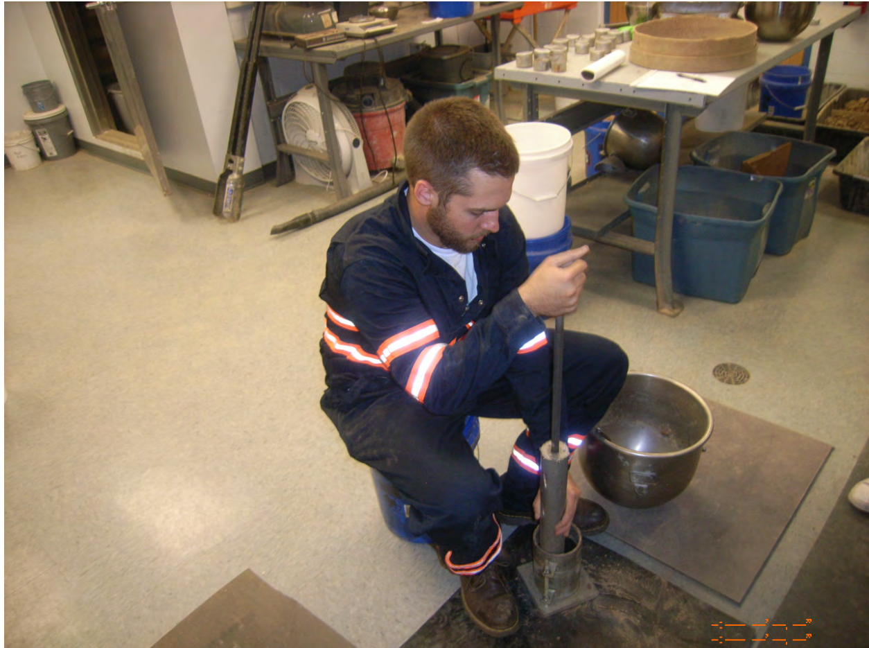
Figure 32: Compaction Mold and Hammer
