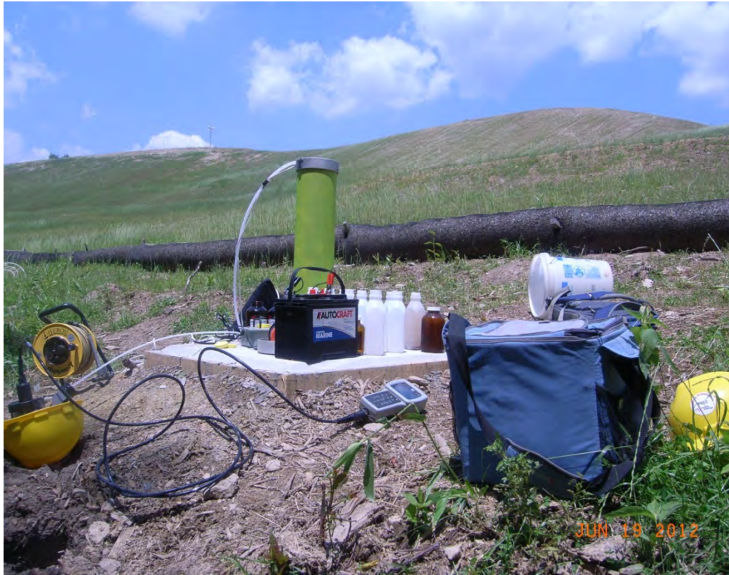
Figure 20: Low Flow Sampling at SHL3 Groundwater Monitoring Well
