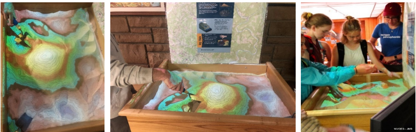
The Augmented Reality Sandbox: A computer projector overlays an interactive topographic map onto sand. By modifying the sand, visitors learn how geomorphologic processes change a landscape and how that landscape is represented on a topographic map
