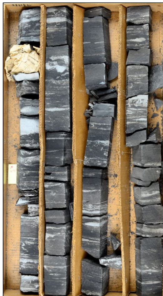
Figure: Example of a box of core containing the Rogersville Shale in a well from Wayne County, West Virginia.
