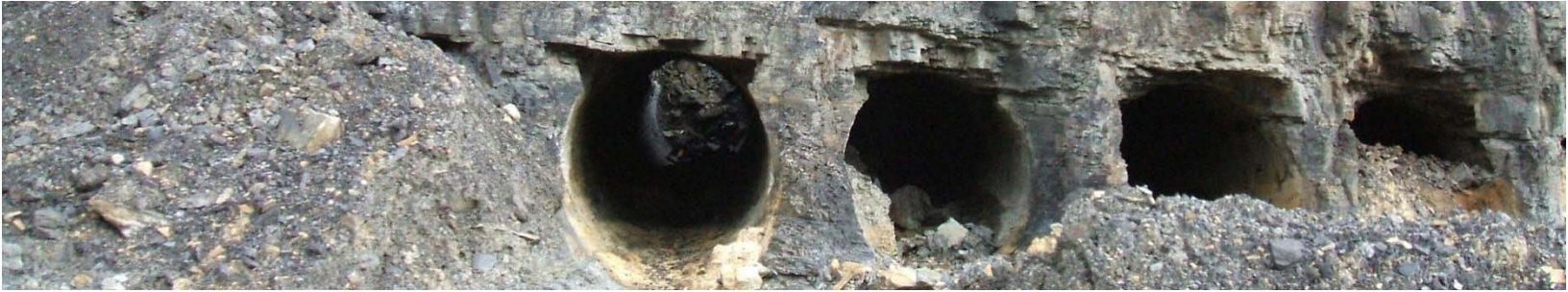
Auger mining for coal (Photo by J. Britton)
