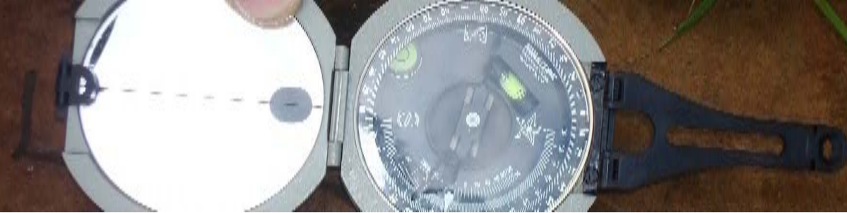
Geologist measuring strike and dip with a Brunton compass (Photo by B. Nugent)
